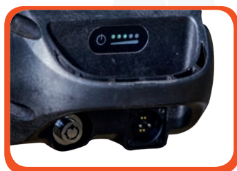
Rosenberg connector with battery indication
