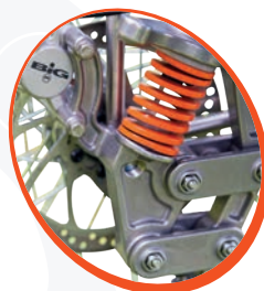
Suspension and hydraulic brakes
